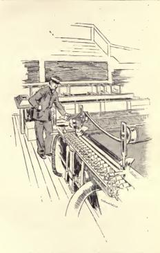
THE PULP FLOWING ON TO MAKING MACHINE.
